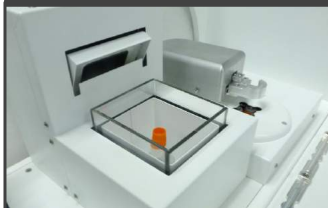
5-Place Automated Balance with XL Series Vial Handler
