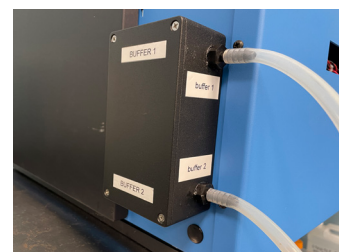
Dual buffer capability: Valve box switches buffers in the protocol
