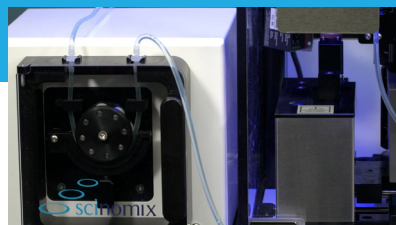
Self-contained, flexible tubing reduces the risk of cross-contamination
