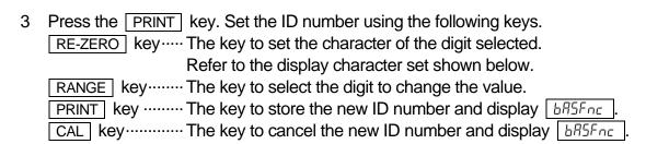
4 With b85Fnc displayed, press the CAL key to return to the weighing mode.
