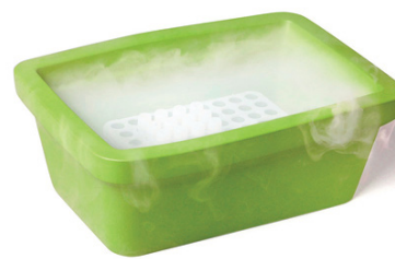
Thermoconductive Tube Rack method: Liquid nitrogen (LN2)
