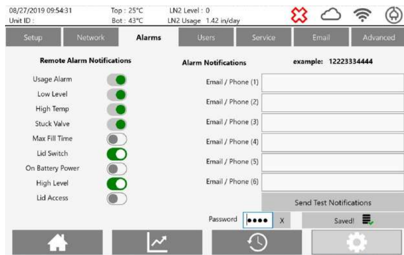
Figure 6-4: Alarm Notifications: local audio/visual, remote text and email, dry alarm contacts
